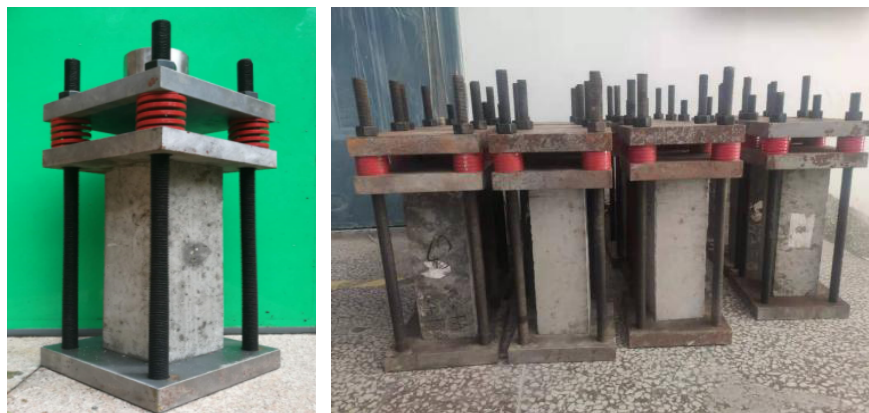
Figure 1: Diagram and physical image of the self-made long-term load device.
