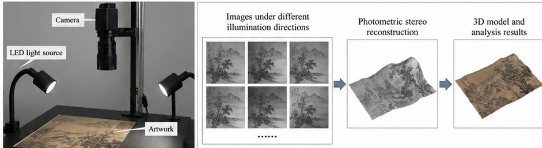
Figure 1: Schematic workflow of photometric stereo for artwork surface inspection
